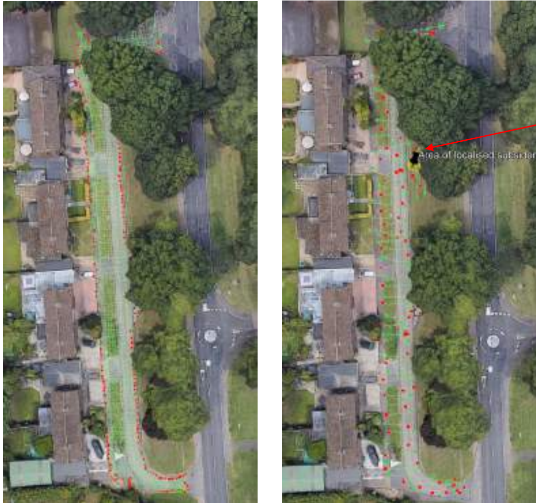
The image on the left (Fig1.) shows the coverage achieved with the 400MHz multi-channel raptor radar system, and the image on the right (Fig2.) is the 270MHz radar antennae coverage.
