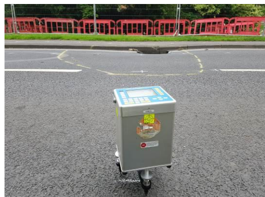
Plate 5 – Microgravity meter at a survey station.
